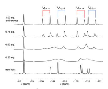
Fig. 2 Sections of the <sup>19</sup>F NMR spectra (471 MHz) of compound 2 and its titration with TBAI in THF-d<sub>8</sub>. Depicted are the signals of the CF<sub>3</sub>groups (left) and the CF2-groups (right, intensities not in the corresponding ratio). Titration experiments of 2 with TMACl and TBABr show a similar pattern (see ESI†).
