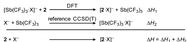
Scheme 4 Isodesmic reactions of host 2 with halides X - (X = F, Cl, Br, I). Enthalpies of formation of the adducts are provided in Table 1, those of the calibration complexes [\text{Sb}(\text{CF}_3)_3 \cdot \text{X}]^- are provided in the ESI† of our previous work. 58
