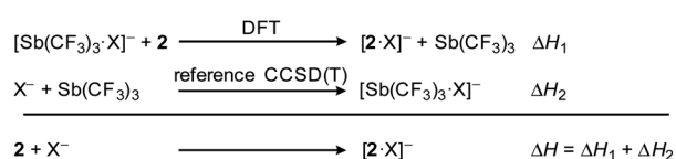
Scheme 4 Isodesmic reactions of host 2 with halides X - (X = F, Cl, Br, I). Enthalpies of formation of the adducts are provided in Table 1, those of the calibration complexes [Sb(CF 3 ) 3 X] - are provided in the ESI† of our previous work. 58
