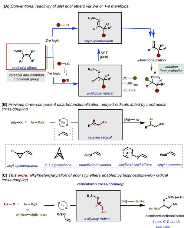
Fig. 1 (A) Traditional strategies based on monocarbofunctionalization of silyl enol ethers *via* 1-e and 2-e enolate-type chemistry. (B) Representative examples of iron-catalyzed dicarbofunctionalization. (C) This work: bisphosphine-iron-catalyzed radical cross-coupling of  $\alpha$ -silyloxy radicals.
