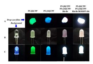
Fig. 7 (A) Drop-cast films; (B) photographs of uncoated LED bulb and coated LED bulb before illumination; (C) photographs of uncoated LED bulb and coated LED bulb after illumination
