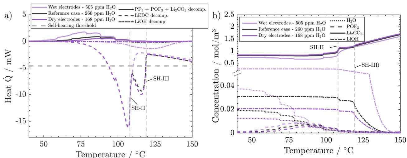
Fig. 7 Effect of H<sub>2</sub>O impurities on behaviour during the ARC test: (a) combined endothermic heat of decomposition of PF<sub>5</sub>, POF<sub>3</sub>, and Li<sub>2</sub>CO<sub>3</sub>, vs. exothermic heat of LEDC and LiOH decomposition. (b) Concentrations of H<sub>2</sub>O, POF<sub>3</sub>, Li<sub>2</sub>CO<sub>3</sub>, and LiOH. Conditions: 45 vol% LEDC, 50 nm SEI.
