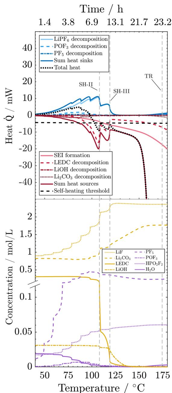
Fig. 4 Processes during the ARC test for the reference case: evolution of heat sinks (blue) and heat sources (red) and related concentrations, as well as the total heat (black) and the self-heating threshold (horizontal dashed line). Vertical dashed lines indicate events marked in Fig. 2. The y-axis break is at  $0.12 \text{ mol m}^{-3}$ .
