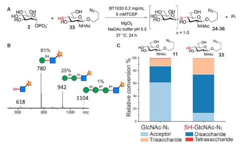
Fig. 3 (A) BT1033 turnover of thio-GlcNAc-N<sub>3</sub> 33 to produce the Manβ1,4-S-GlcNAc-N<sub>3</sub> 34 thioglycoside. Reaction mechanism depicted in the reverse phosphorolysis direction. (B) LC-MS analysis showing di-, tri- and tetrasaccharide thioglycoside formation. (C) Comparative product distribution in BT1033 reactions with 11 and 33
