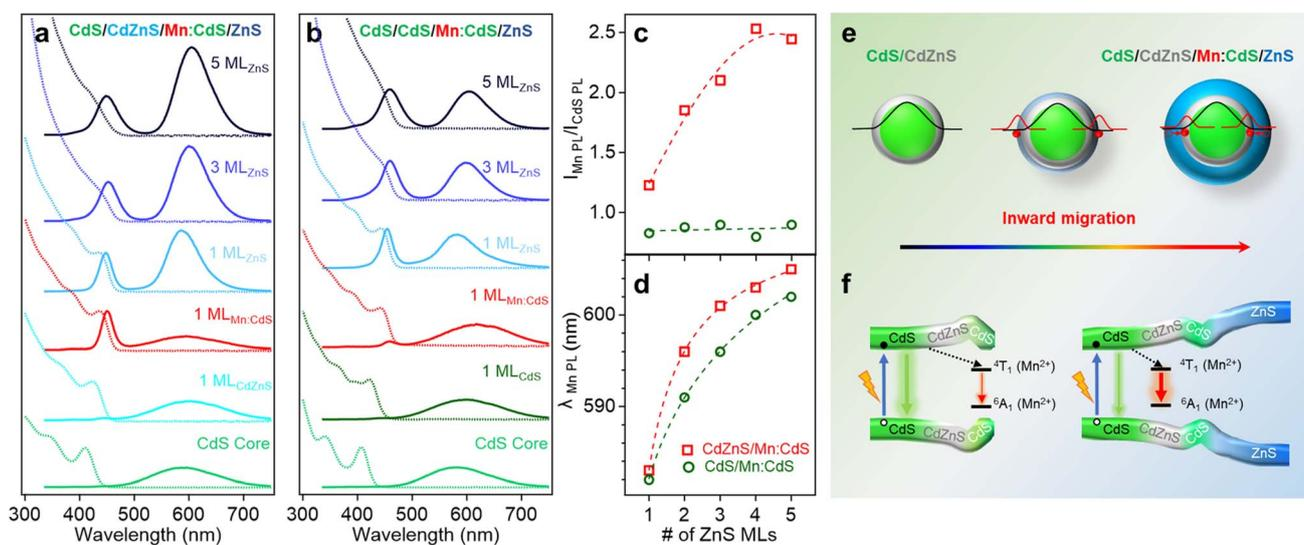
Fig. 5 (a and b) Normalized absorption and PL spectra of (a) CdS/CdZnS/Mn:CdS/ZnS<sub>(1–5 MLs)</sub> and (b) CdS/CdS/Mn:CdS/ZnS<sub>(1–5 MLs)</sub> core/multi-shell QDs. (c) The PL Intensity ratio of Mn(II) and CdS host lattice and (d) the changes of Mn(II) PL peak position as a function of ZnS shell thickness. (e) Schematic of the dopant inward migration by inserted CdZnS alloyed trap layer and (f) the band alignment of the CdS/CdZnS/Mn:CdS/ZnS core/multi-shell QDs.
