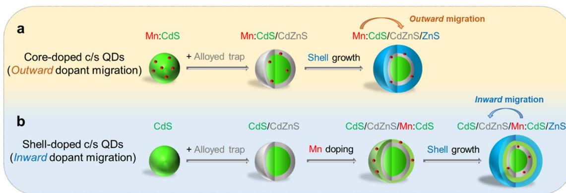
Scheme 1 Schematic of (a) core-doped and (b) shell-doped core/multi-shell QDs with directional (outward and inward) dopant migration by inserting an alloyed “trap” for Mn dopants.
