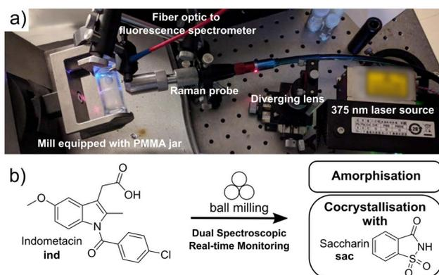
Fig. 1 (a) Instrumental setup for tandem time-resolved *in situ* monitoring of milling reactions using solid-state fluorescence emission and Raman spectroscopies. (b) Model mechanochemical transformations monitored in this work: amorphisation and cocrystallisation of indometacin (**ind**).
