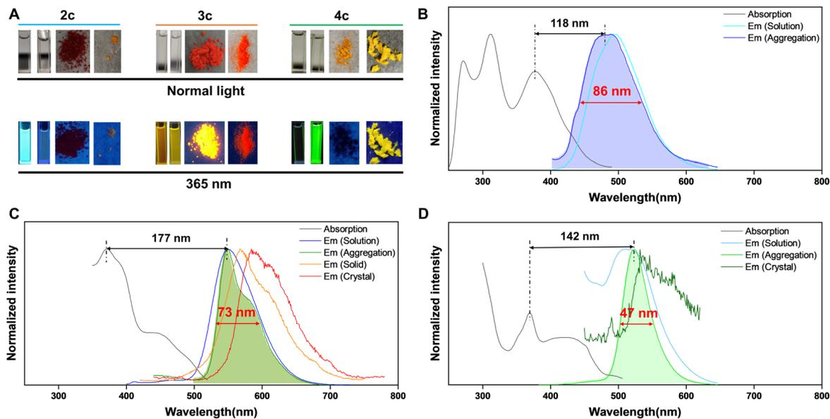
Fig. 2 Luminescence properties of **2c**, **3c**, and **4c**. (A) Photos of compounds **2c**, **3c**, and **4c** (from left to right: solution, aggregation, solid, and crystal state) under normal light (up) and 365 nm UV light (down). Normalized absorption and PL spectra of **2c** (B), **3c** (C), and **4c** (D) in different states. Concentration: 10  $\mu\text{M}$ .
