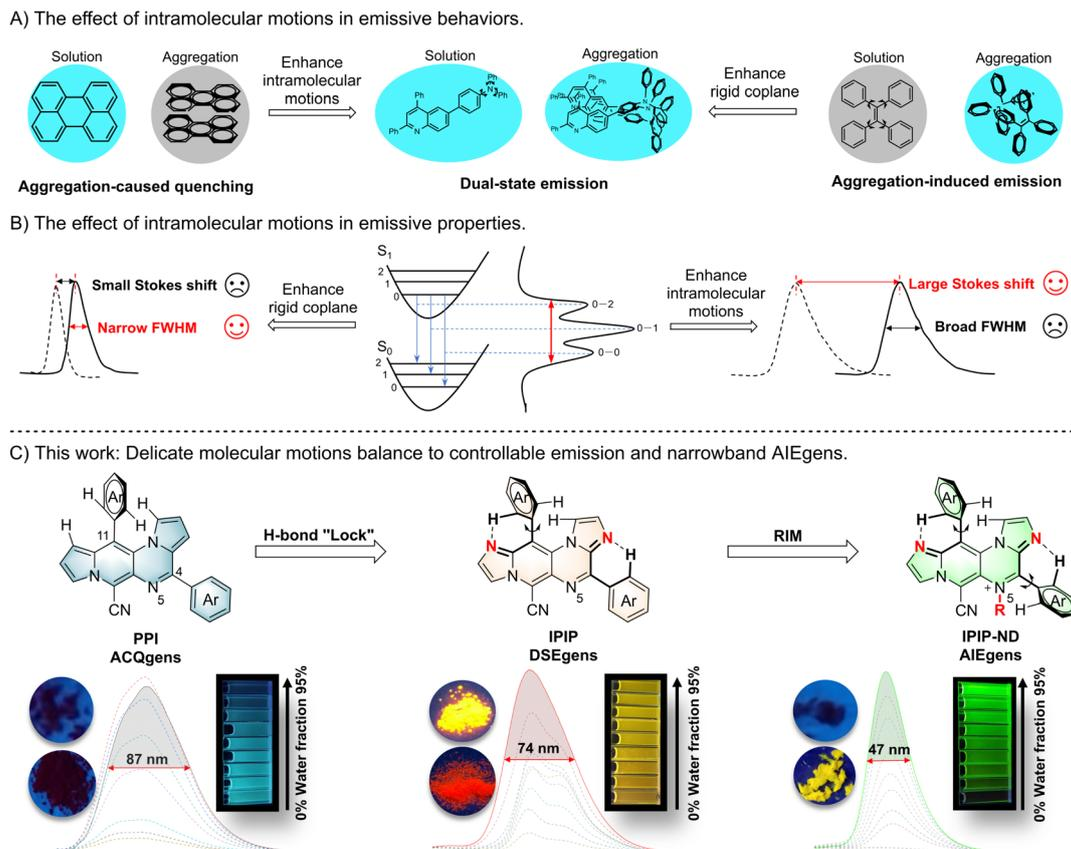
Fig. 1 Effect of intramolecular motion on the emissive behavior (A) and properties (B) of fluorescent molecules, and the discovery of controllable ideal aza-dicyclopenta[*a,g*]naphthalene luminogens *via* delicate balance of intramolecular motions (C).
