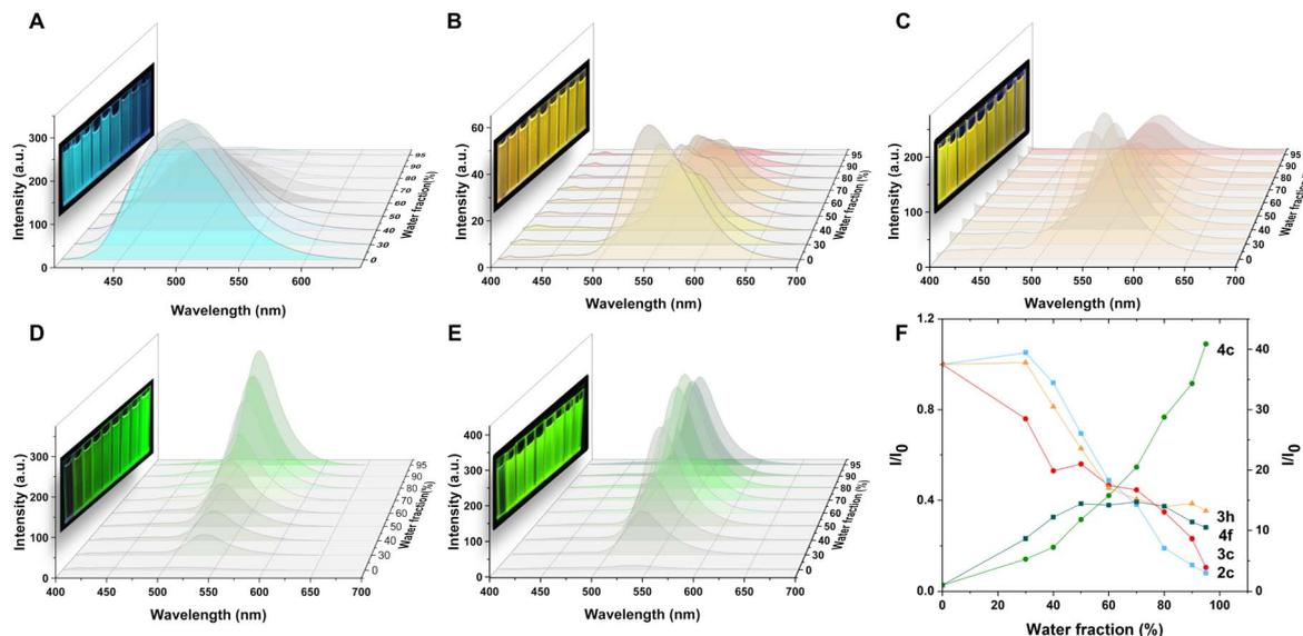
Fig. 3 Emission spectra of **2c** (A), **3c** (B), **3h** (C), **4c** (D), **4f** (E), and (F) plots of emission intensity  $I/I_0$  of **2c** (496 nm, blue line), **3c** (550 nm, red line), **3h** (551 nm, orange line), **4c** (524 nm, light green line), and **4f** (533 nm, deep green line) in different water fractions (inset: photos of **2c**, **3c**, **3h**, **4c**, and **4f** in various water fractions under 365 nm UV light). Concentration: 10  $\mu\text{M}$ .
