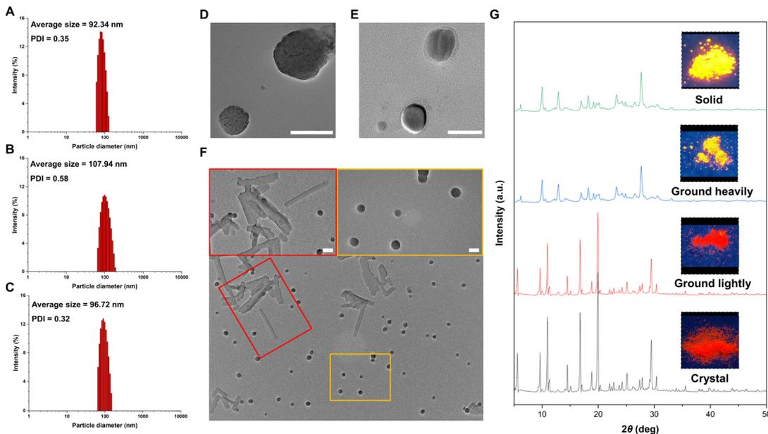
Fig. 4 DLS size distribution of **2c** (A), **3c** (B), and **4c** (C) in 95% water/5% DMSO; TEM of **2c** (D), **4c** (E), and **3c** (F) in 95% water/5% DMSO; powder X-ray diffraction patterns of **3c** (G) in different states (scale bar: 100 nm).
