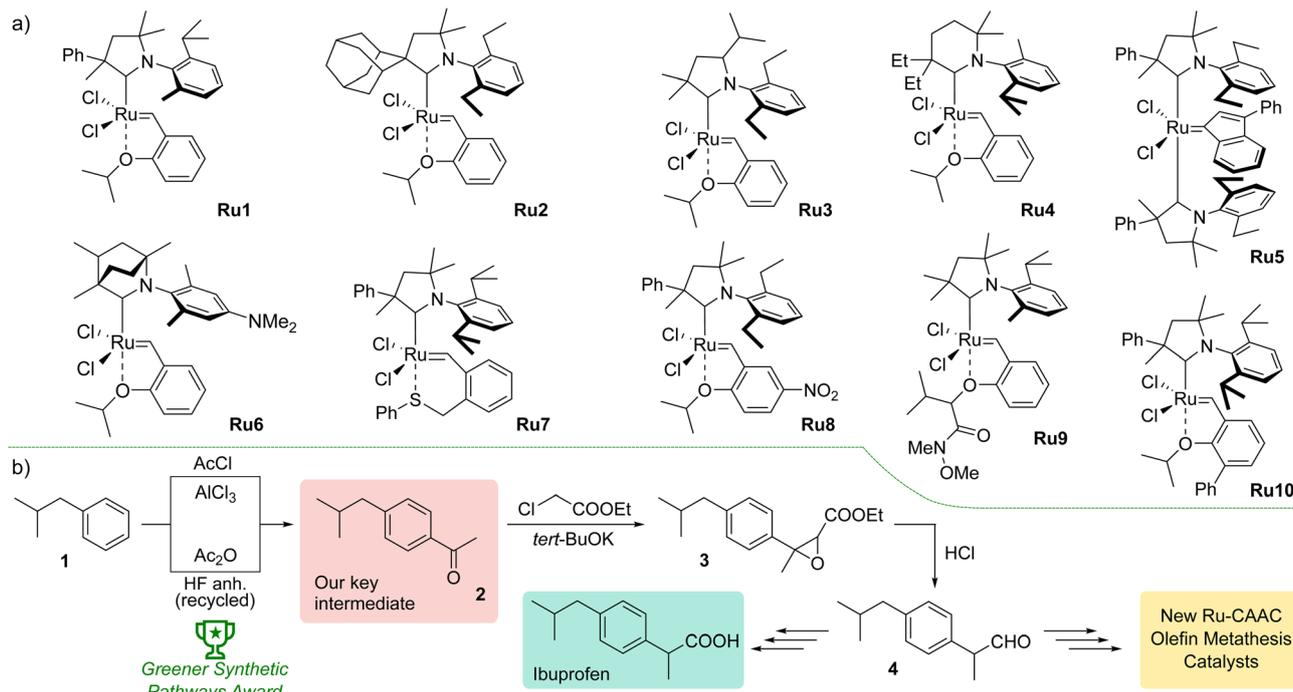
**Fig. 1** (a) Examples of CAAC-based ruthenium complexes showing diverse structural modifications of the CAAC ligand structure. (b) Upper path, original synthetic pathway to Ibuprofen by Boots UK Limited. Lower path, currently used Friedel–Crafts acylation optimised to meet *Green Chem.* principles.
