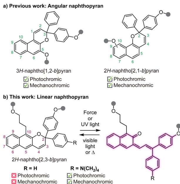
**Scheme 1** Naphthopyran isomers and their stimuli-responsive behavior. (a) Angular naphthopyrans undergo ring-opening reactions with UV light or mechanical force. (b) Photochromism and mechanochromism of linear 2H-naphthopyran is enabled upon introduction of an electron donating dialkylamine substituent.
