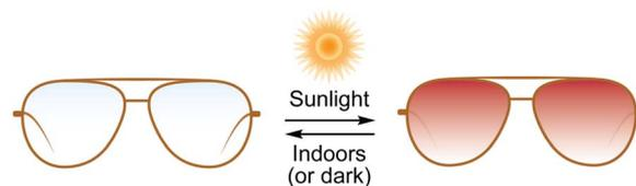
Fig. 5 Naphthopyrans have been developed extensively as UV light-responsive coloring (*i.e.*, photochromic) agents in plastic ophthalmic lenses.
