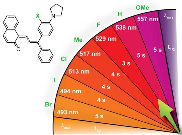
Fig. 7 Merocyanine color can be finely tuned by modulating the steric demand of the group adjacent to a *para*-pyrrolidine substituent. The  $\lambda_{\max}$  and half-life ( $t_{1/2}$ ) are given for merocyanines with various *meta*-substituents (X). Values shown were measured in toluene at 20 °C.<sup>214</sup>
