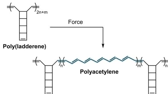
Scheme 2 Poly(ladderene) undergoes a force-induced unzipping reaction to produce conjugated polyacetylene.
