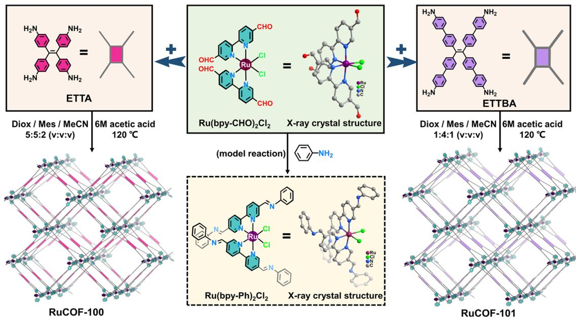
Fig. 1 The synthetic procedures for model compounds  $\text{Ru}(\text{bpy-Ph})_2\text{Cl}_2$ ,  $\text{RuCOF-100}$  and  $\text{RuCOF-101}$ , respectively. The corresponding X-ray single crystal structures of metal complex building unit  $\text{Ru}(\text{bpy-CHO})_2\text{Cl}_2$  and model compound  $\text{Ru}(\text{bpy-Ph})_2\text{Cl}_2$  are shown, in which all H atoms and solvent molecules have been removed for clarity.
