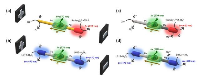
Scheme 1 Schematic illustration of the different hybrid wireless light-emitting systems used for (a and b) the exogenous and (c and d) endogenous bipolar electrochemistry approach, with a representation of the associated chemical reactions, the electron flux and the color of the resulting light emissions.
