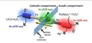
Scheme 2 Schematic illustration of the divided light-emitting bipolar system used for the endogenous multimodal approach, with a representation of the associated chemical reactions, the electron flux, the physical separation, the ionic conductor (dot lines) and the cathodic (blue)/LED (green)/anodic (red) light emissions.
