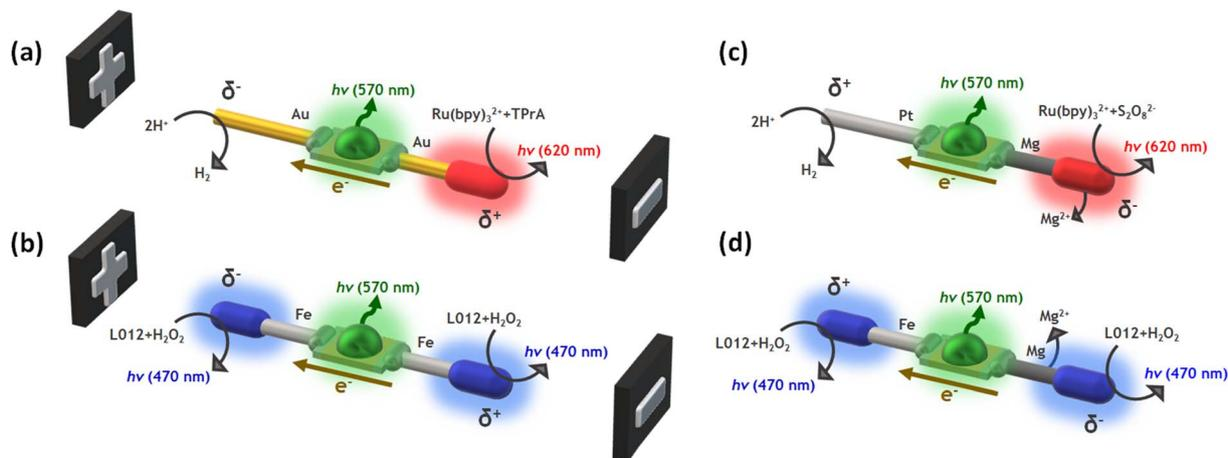
**Scheme 1** Schematic illustration of the different hybrid wireless light-emitting systems used for (a and b) the exogenous and (c and d) endogenous bipolar electrochemistry approach, with a representation of the associated chemical reactions, the electron flux and the color of the resulting light emissions.
