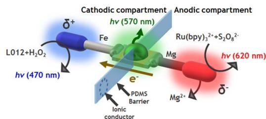
**Scheme 2** Schematic illustration of the divided light-emitting bipolar system used for the endogenous multimodal approach, with a representation of the associated chemical reactions, the electron flux, the physical separation, the ionic conductor (dot lines) and the cathodic (blue)/LED (green)/anodic (red) light emissions.
