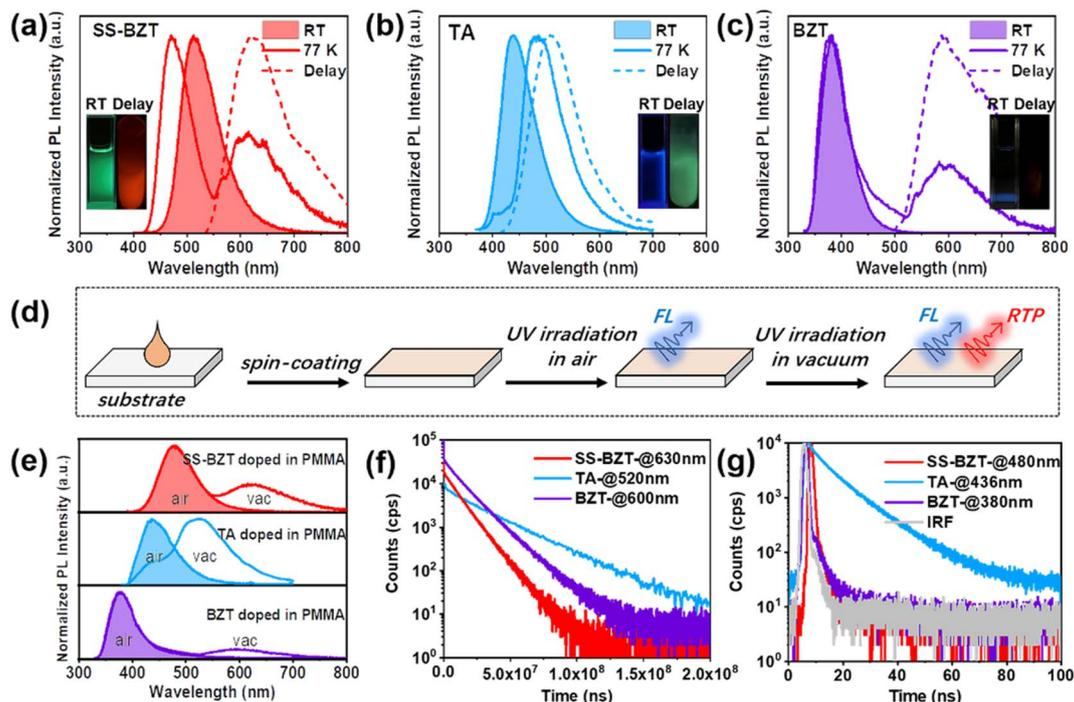
Fig. 3 PL spectra (conditions: RT and 77 K) and gated PL spectra (delay time: 1 ms) of (a) SS-BZT, (b) TA, and (c) BZT dispersed in THF solution at  $10^{-5}$  mol L $^{-1}$ . (d) Schematic of luminescence from doped PMMA film. (e) PL spectra of 1.00 wt% doped PMMA films for SS-BZT, TA, and BZT at RT (in air and vacuum). (f) and (g) Time-resolved PL spectra of 1.00 wt% doped PMMA films for SS-BZT, TA and BZT in a vacuum at RT.
