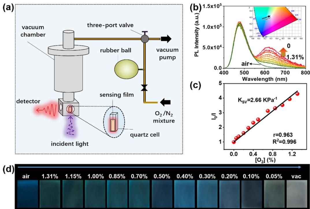
Fig. 5 (a) Schematic of detecting oxygen concentration in this work. (b) PL spectra and (c) plot of  $I_0/I$  against  $[O_2]$  of 1.00 wt% SS-BZT-doped PMMA film at different  $[O_2]$ . Inset shows CIE coordinates corresponding to the PL spectra with decreasing  $[O_2]$  of 1.00 wt% SS-BZT-doped PMMA film. (d) Images of 1.00 wt% SS-BZT-doped PMMA film under 365 nm irradiation with decreasing  $[O_2]$ .
