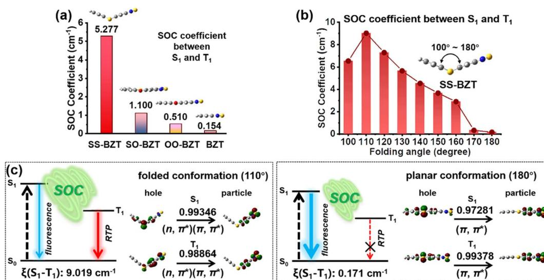
Fig. 4 (a) Molecular conformations and SOC coefficients for  $S_1-T_1$  based on the molecular geometries of SS-BZT, SO-BZT, OO-BZT, and BZT in crystals. (b) SOC coefficients for  $S_1-T_1$  based on the molecular geometries of the SS-BZT crystal at different folding dihedral angles. (c) Schematic of folding-induced SOC enhancement and NTOs of  $S_1$  and  $T_1$  states for SS-BZT in a folded conformation ( $110^\circ$ ) and planar conformation ( $180^\circ$ ).
