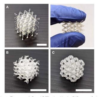
Fig. 4 Thermosets A, B, and C 3D-printed by the CLIP system. Scale bar  $= 1 \ \text{cm}.$
