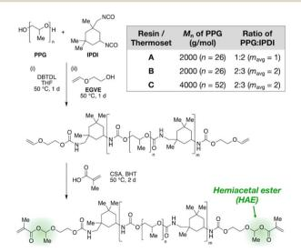
Fig. 2 Tunable synthetic design of HAE-based photopolymerizable polyurethanes. DBTDL, dibutyltin dilaurate; CSA, rac-camphorsulfonic acid; BHT, butylated hydroxytoluene. Inset table: composition of Resins/Thermosets A, B, and C studied in this work.
