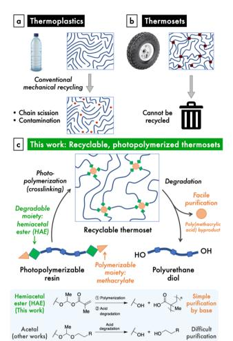
Fig. 1 (a) Conventional mechanical recycling of thermoplastics remains a limited solution to plastic waste. (b) Thermosets are covalently crosslinked and thus impossible to reprocess or recycle. (c) In this work, we report a modular design for a degradable and recyclable photopolymerized thermoset based on chemically labile hemiacetal ester (HAE) linkages and polyurethane backbones. The HAE linkage enables facile purification after mild acid degradation.
