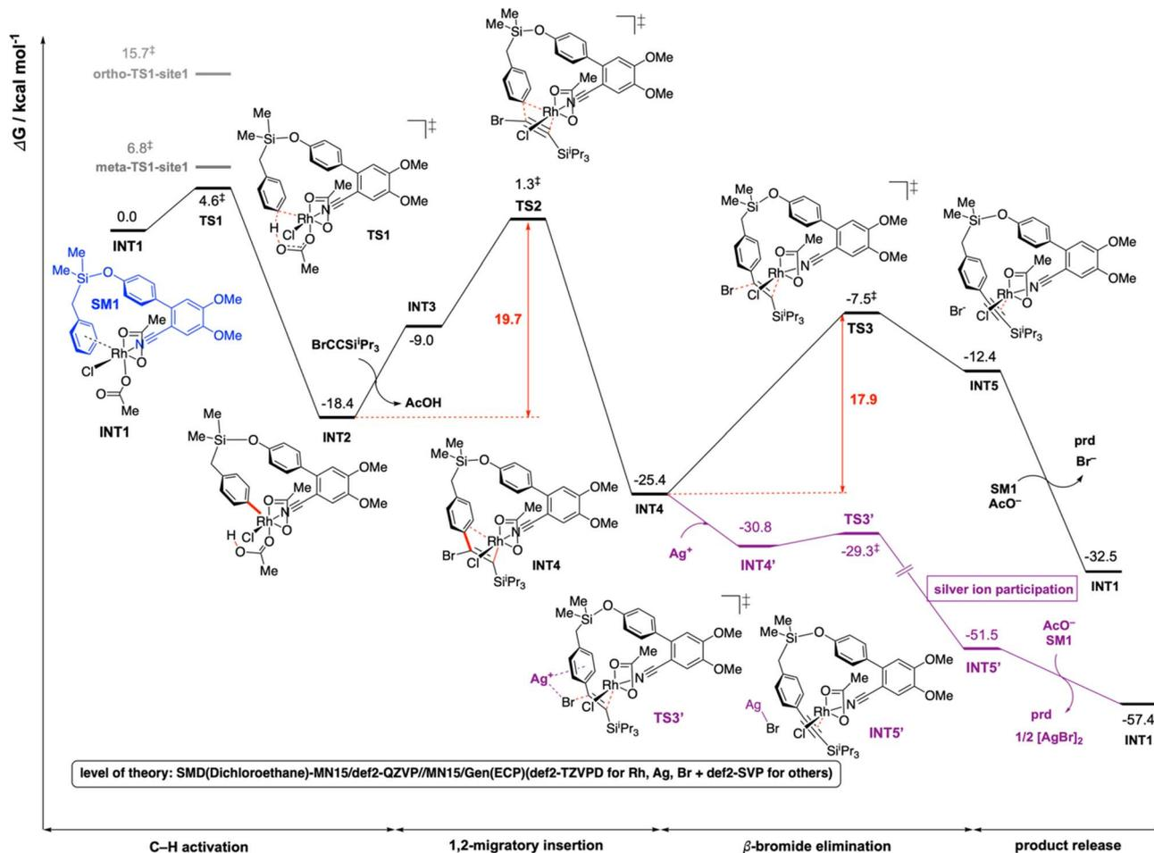
Fig. 1 Gibbs energy profile for the Rh-catalyzed C(sp<sup>2</sup>)-H alkylation of arenes. DFT optimized key transition structures are shown in Fig. 2.
