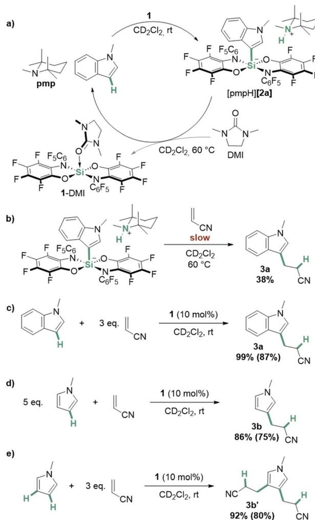
Fig. 4 Schematic depiction of (a) the synthesis of  $[\text{pmpH}][\mathbf{2a}]$  from *N*-methylindole and the reverse reaction triggered by DMI, (b) the reaction of acrylonitrile and  $[\text{pmpH}][\mathbf{2a}]$ , the addition of (c) *N*-methylindole and (d)/(e) *N*-methylpyrrole to acrylonitrile catalyzed by **1**. Yields were determined against cyclooctane as an internal standard, yields in parentheses are isolated yields (details see ESI†).
