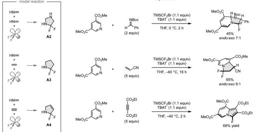
Fig. 13 Experimental realization based on computationally predicted three-component reactions. (a) Realization of the predicted reaction with the support of additional DFT calculations at the  $\omega$ B97X-D/Def2-SVP/CPCM(THF) level. (b) Further experimental demonstrations.
