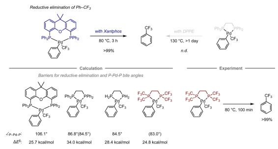
Fig. 6 Computational design of phosphine ligands for the reductive elimination of benzotrifluoride from Pd complexes; calculations were performed at the ONIOM(B3LYP/6-31+G(d) (with LANL2DZ for Pd): HF/LANL2MB) level. The bite angles shown in parentheses were calculated at the B3LYP/6-31+G(d,p) (with LANL2DZ for Pd) level.
