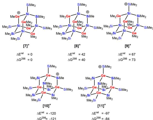
Fig. 4 Relative energies  $\Delta E^{\text{rel}}$  and free enthalpies  $\Delta G^{298}$  of  $\text{Si}_{10}\text{Ge}_4\text{-Me}_{23}$  cations derived from heteroadamantanes 3 ([7]<sup>+</sup>–[9]<sup>+</sup>) and 4 from ([10]<sup>+</sup>, [11]<sup>+</sup>), in  $\text{kJ mol}^{-1}$ , at M06-2X/6-311+G(d,p).
