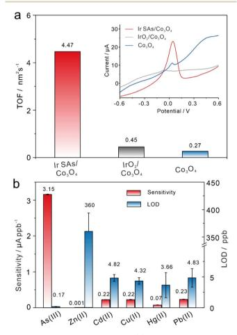
Fig. 2 Electrochemical detection of As(III) and selectivity tests toward common heavy metal ions. (a) Comparison of TOF and LSV responses toward 10 ppb As(III) (inset) on Ir SAs/ $Co_3O_4$ , Ir $O_2/Co_3O_4$ , and  $Co_3O_4$ modified electrodes under the same conditions. (b) Sensitivity and LOD of Ir SAs/Co<sub>3</sub>O<sub>4</sub> toward different HMIs.
