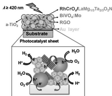
Fig. 5 Schematic of a-TiO<sub>2</sub>-coated (RhCrO<sub>x</sub>/ZrO<sub>2</sub>/LaMg<sub>1/3</sub>Ta<sub>2/3</sub>O<sub>2</sub>N)/(Au, RGO)/BiVO<sub>4</sub>:Mo photocatalyst sheet. Adapted with permission from ref. 44. Copyright 2016 Wiley-VCH.
