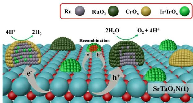
Fig. 8 Schematic of dispersion of cocatalysts and dominant charge transfer processes on the SrTaO<sub>2</sub>N surface. Adapted with permission from ref. 57. Copyright 2023 American Chemical Society.
