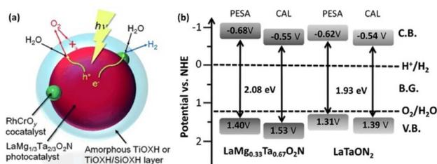
Fig. 6 (a) Schematic of the OWS reaction mechanism on surface-coated RhCrO<sub>x</sub>/LaMg<sub>1/3</sub>Ta<sub>2/3</sub>O<sub>2</sub>N. Adapted with permission from ref. 46. Copyright 2015 Wiley-VCH. (b) Band levels for LaMg<sub>x</sub>Nb<sub>1-x</sub>O<sub>1+3x</sub>N<sub>2-3x</sub> (*x* = 0 and 0.33) estimated by theoretical calculations (CAL) and photoelectron spectroscopy in air (PESA). Adapted with permission from ref. 47. Copyright 2016 The Royal Society of Chemistry.
