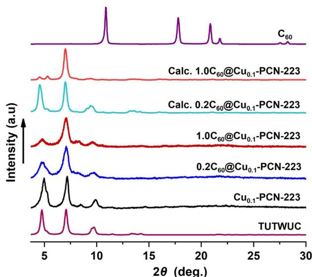
Fig. 2 PXRD data for Cu<sub>0.1</sub>-PCN-223 and the C<sub>60</sub>@Cu<sub>0.1</sub>-PCN-223 composites vs. PXRD data for PCN-223 simulated from the single crystal diffraction data (Cambridge Crystallographic Data Centre (CCDC) code: TUTWUC) and two fulleretic composites optimized in this study (please see Section 2.2).
