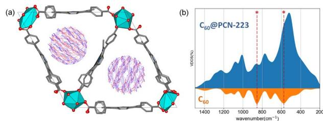
Fig. 3 (a) Superposition of time-averaged snapshots for  $C_{60}$  within a 100 ps time-window of  $C_{60}@PCN-223$  dynamics at DFTB level of theory. (b) MD recovered the total and projected vibrational density of states for  $C_{60}@PCN-223$  and  $C_{60}$ , where asterisks mark the most profound contribution by  $C_{60}$  in the total VDOS.
