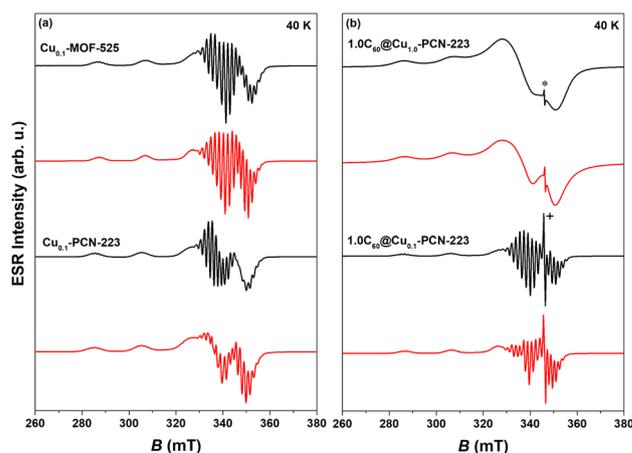
Fig. 5 Experimental (black) and simulated CW-ESR spectra (red) of various MOFs recorded at 40 K: (a)  $\text{Cu}_{0.1}\text{-MOF-525}$  and  $\text{Cu}_{0.1}\text{-PCN-223}$ , (b)  $1.0\text{C}_{60}\text{@Cu}_{0.1}\text{-PCN-223}$  and  $1.0\text{C}_{60}\text{@Cu}_{0.1}\text{-PCN-223}$ . Asterisk in the figure indicates the fullerene-radical (FR) signal at  $g \approx 2.003$  while "+" denotes truncation of the peak. Parameters of the simulated spectra are reported in Table S1.†
