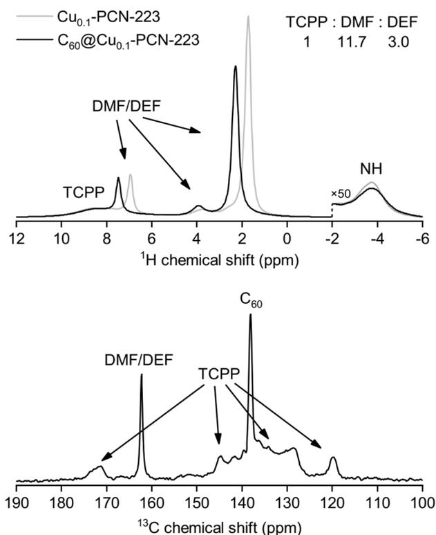
Fig. 4 (Up)  $^1\text{H}$  MAS NMR spectra for  $\text{Cu}_{0.1}\text{-PCN-223}$  and  $1.0\text{C}_{60}\text{@Cu}_{0.1}\text{-PCN-223}$  at 300 K. (Down)  $^{13}\text{C}$  MAS NMR spectrum of  $1.0\text{C}_{60}\text{@Cu}_{0.1}\text{-PCN-223}$  at 300 K. The signals from dimethylformamide (DMF), diethylformamide (DEF),  $\text{H}_2\text{TCPP}$  linker and fullerene ( $\text{C}_{60}$ ) are indicated on the spectra.
