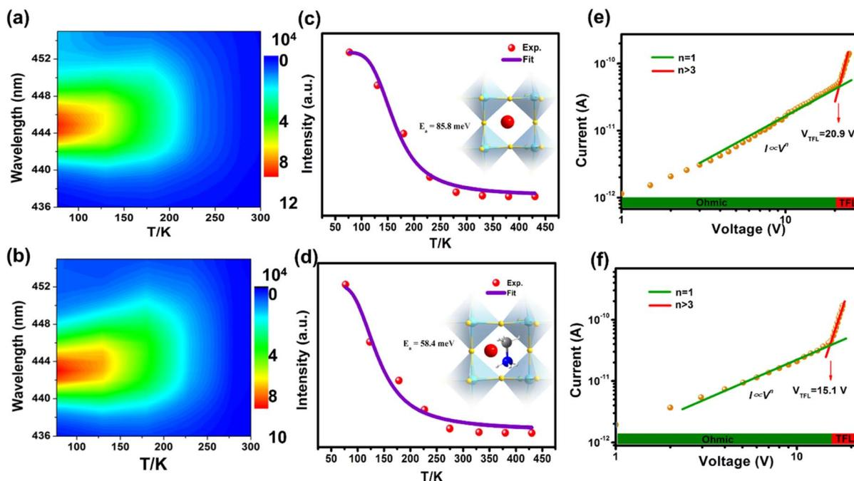
Fig. 3 Possible origin of strong FPP effects in the  $\text{BA}_2\text{Cs}_{1-x}\text{MA}_x\text{Pb}_2\text{Br}_7$  family. Contour plots of the temperature-dependent PL emission spectra of  $x = 0$  (a) and  $x = 0.34$  (b) in the temperature range of 77–300 K. Exciton binding energy determination of  $x = 0$  (c) and  $x = 0.34$  (d). The trap density measurements for single crystals of  $x = 0$  (e) and  $x = 0.34$  (f), respectively.
