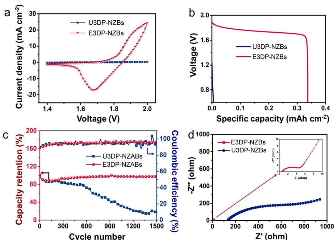
Fig. 4 Comparison between U3DP-NZABs and E3DP-NZABs. (a) CV curves at a scan rate of  $10 \text{ mV s}^{-1}$ . (b) Galvanostatic discharge curves at a current density of  $1.2 \text{ mA cm}^{-2}$ . (c) Long-term cycling performance. (d) EIS curves.
