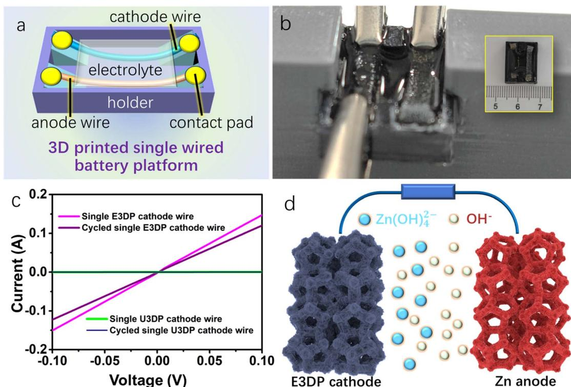
Fig. 3 (a) Schematic of 3D printed single-wired battery measurement devices. (b) Photograph of measurement platform devices. (c) *I*-*V* results of various 3D printed single cathode wires before and after electrochemical cycles. (d) Schematic of the charge storage mechanism of NZABs.
