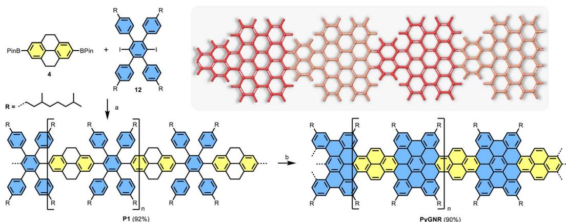
Scheme 2 Synthetic route to **PyGNR**. Reagents and conditions: (a) **4** (stoichiometric), **12**, Pd(PPh<sub>3</sub>)<sub>4</sub>, K<sub>2</sub>CO<sub>3</sub>, Aliquat 336, PhMe/H<sub>2</sub>O, 110 °C, 48 h; (b) FeCl<sub>3</sub>, MeNO<sub>2</sub>, CH<sub>2</sub>Cl<sub>2</sub>, rt, 7 d. Inset is the optimized geometry of **PyGNR**, aliphatic side chains omitted for clarity.
