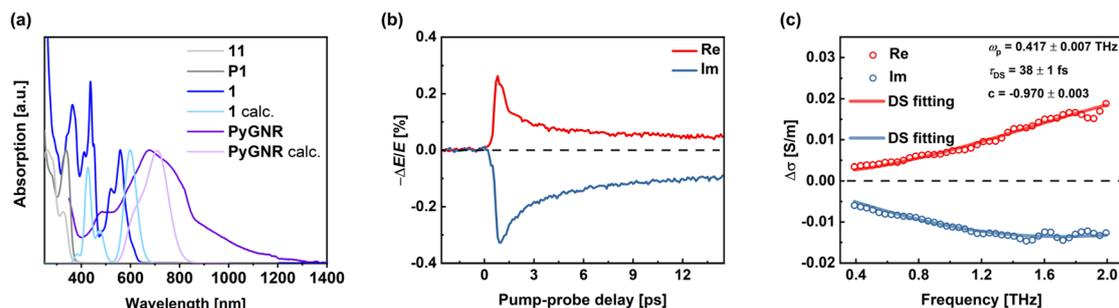
Fig. 6 (a) Absorption spectra of 1, 11, P1 (CHCl<sub>3</sub>), and PyGNR (NMP) as well as DFT-predicted 1 and PyGNR; (b) time-resolved terahertz photoconductivity of PyGNR following photoexcitation. The absorbed photon fluence is  $\sim 1$  mJ cm<sup>-2</sup>. (c) The frequency-resolved THz complex conductivity measured  $\sim 1.2$  ps after photoexcitation. The solid lines are fits to the Drude–Smith model.
