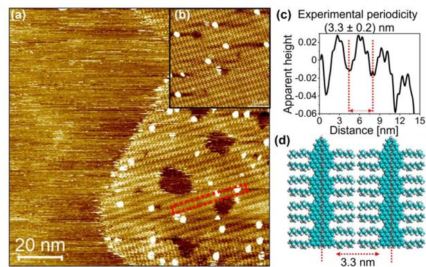
Fig. 5 Large scale (a) and high resolution (b) STM images of **PyGNR** self-assembled at the heptanoic acid/HOPG interface; (c) graphite-calibrated representative line-profile measured along the red arrow direction in STM image of panel (a); (d) molecular model of **PyGNR** showing packing without alkyl chain interdigitation.  $U_{\text{bias}} = -0.4\text{ V}$  and  $I_{\text{set}} = 0.05\text{ nA}$ .
