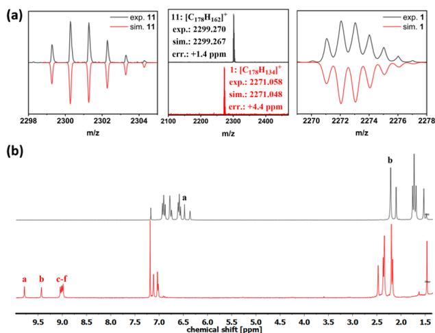
Fig. 2 (a) MALDI-TOF-MS of compounds **11** and **1**. (b) <sup>1</sup>H-NMR spectra of compound **11** (top) and compound **1** (bottom), recorded in CDCl<sub>3</sub> at 300 MHz (proton labels see Scheme 1).
