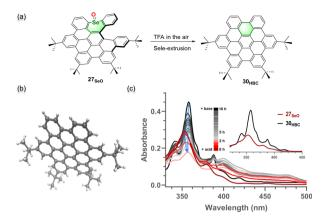
Fig. 5 (a) Acid-catalyzed HBC formation from HBC precursor selenium-doped NG  $27_{SeO}$ . (b) X-ray crystallographic structure of  $30_{HBC}$ with 50% probability of thermal ellipsoids. (c) Changes in the UV-vis absorption spectra of 27<sub>SeO</sub> upon dissolving it in trifluoroacetic acid/ DCM (1/2, v/v) with 3.3 µM concentration under ambient conditions.
