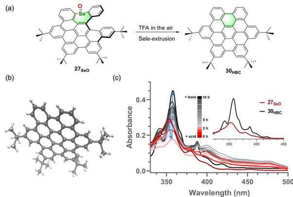
Fig. 5 (a) Acid-catalyzed HBC formation from HBC precursor selenium-doped NG  $27_{\text{SeO}}$ . (b) X-ray crystallographic structure of  $30_{\text{HBC}}$  with 50% probability of thermal ellipsoids. (c) Changes in the UV-vis absorption spectra of  $27_{\text{SeO}}$  upon dissolving it in trifluoroacetic acid/DCM (1/2, v/v) with  $3.3 \mu\text{M}$  concentration under ambient conditions.
