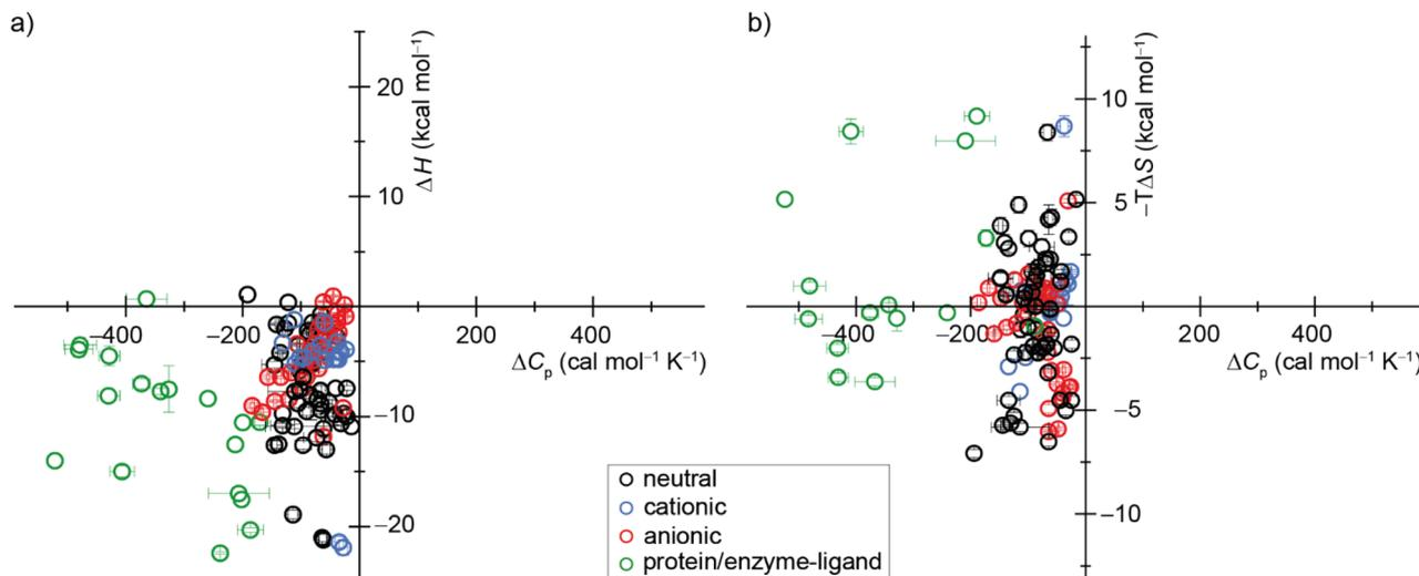
Fig. 7 Display of a scatter plot between host–guest and protein–ligand (a) binding enthalpies ( $\Delta H_{\text{exp}}$ ) and (b) binding entropies ( $-T\Delta S_{\text{exp}}$ ) versus heat capacity changes ( $\Delta C_{p,b}$ ). See ESI, Tables S5 and S6 as well as Fig. S28† for details on the host–guest pairs, experimental conditions, exact values, and references.
