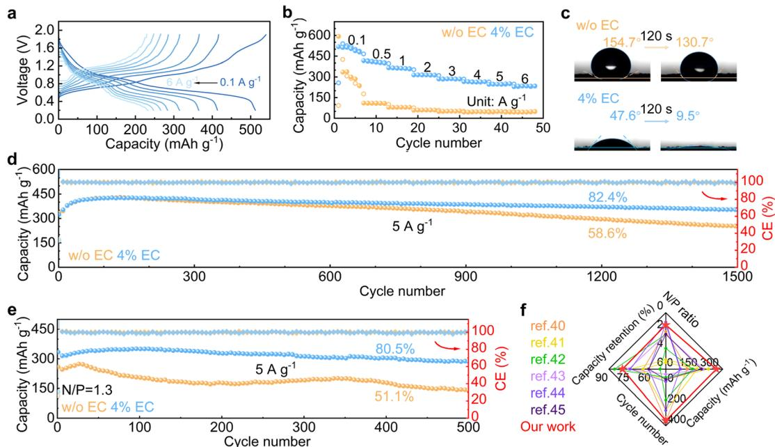
Fig. 6 (a) Charge–discharge curves of the  $V_6O_{13}\cdot H_2O$  cathode in 4% EC and (b) rate performance in the two electrolytes. (c) Contact angles between the electrolytes and cathode before and after 120 s rest. Long-term cycling of  $V_6O_{13}\cdot H_2O$  at  $5 A g^{-1}$  with (d) excess Zn anode and (e) limited Zn anode with  $N/P = 1.3$ . (f) Cycling performance comparison of full cells using limited Zn anodes with previous reports.
