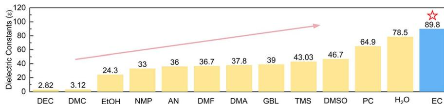
Fig. 1 Dielectric constants of EC and other common solvents including H<sub>2</sub>O.
