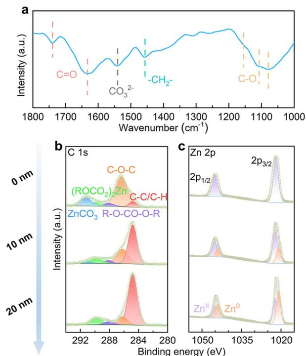
Fig. 3 (a) FT-IR, (b) C 1s and (c) Zn 2p XPS with different sputtering depths by Ar<sup>+</sup> of the Zn electrode after 25 cycles in the 4% EC electrolyte.
