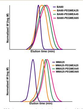
Fig. 6 GPC chromatograms for the chain extensions of BA60 (top) and MMA25 (bottom) with PEGMEA.
