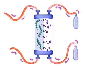
Fig. 1 The general principle of the inline dialysis module used in this work. A polymer is synthesised and brought in continuously *via* the inlet. The unreacted monomer is removed *via* membrane dialysis.
