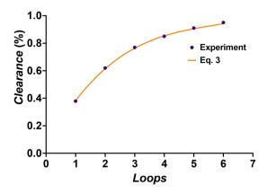
Fig. 5 Comparison of the predicted clearance of the monomer via eqn (3) for pBA-DP60 and the measured progress of clearance via inline NMR
