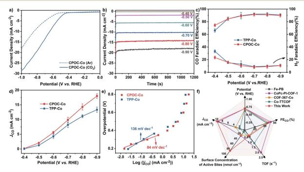
Fig. 3 (a) LSV curves for CPOC-Co. (b) Chronoamperometric responses at different potentials (vs. RHE) for CPOC-Co. (c) Comparison of the faradaic efficiency between CPOC-Co and TPP-Co. (d) Comparison of the partial CO current density between CPOC-Co and TPP-Co. (e) Tafel plots of CPOC-Co and TPP-Co. (f) Comparison of the performance to other electrocatalytic materials.
