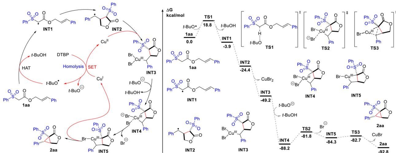
Scheme 2 Proposed mechanism and computed energy profile for the Cu-catalysed intramolecular cyclopropanation of **2aa**. Energies are in kcal mol<sup>-1</sup> and bond distances are labelled in Å.
