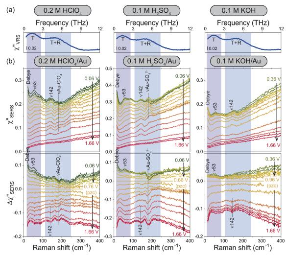
Fig. 2 (a)  $\chi''_{VRS}$  spectra for bulk aqueous solutions containing different electrolytes. (b) Potential dependence of  $\chi''_{SERS}$  spectra for the respective electrolyte solutions on Au surfaces (upper panel) and their  $\Delta \chi''_{SERS}$  spectra with respect to pzc for each solution (bottom).
