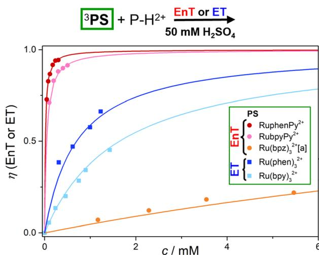
Fig. 5 Comparative quenching efficiency analysis for EnT (color-coded bullets) or ET (color-coded squares) between the excited photosensitizers at a constant concentration of 50 mM H<sub>2</sub>SO<sub>4</sub> (a) in H<sub>2</sub>O due to sensitizer protonation in acidic solution).
