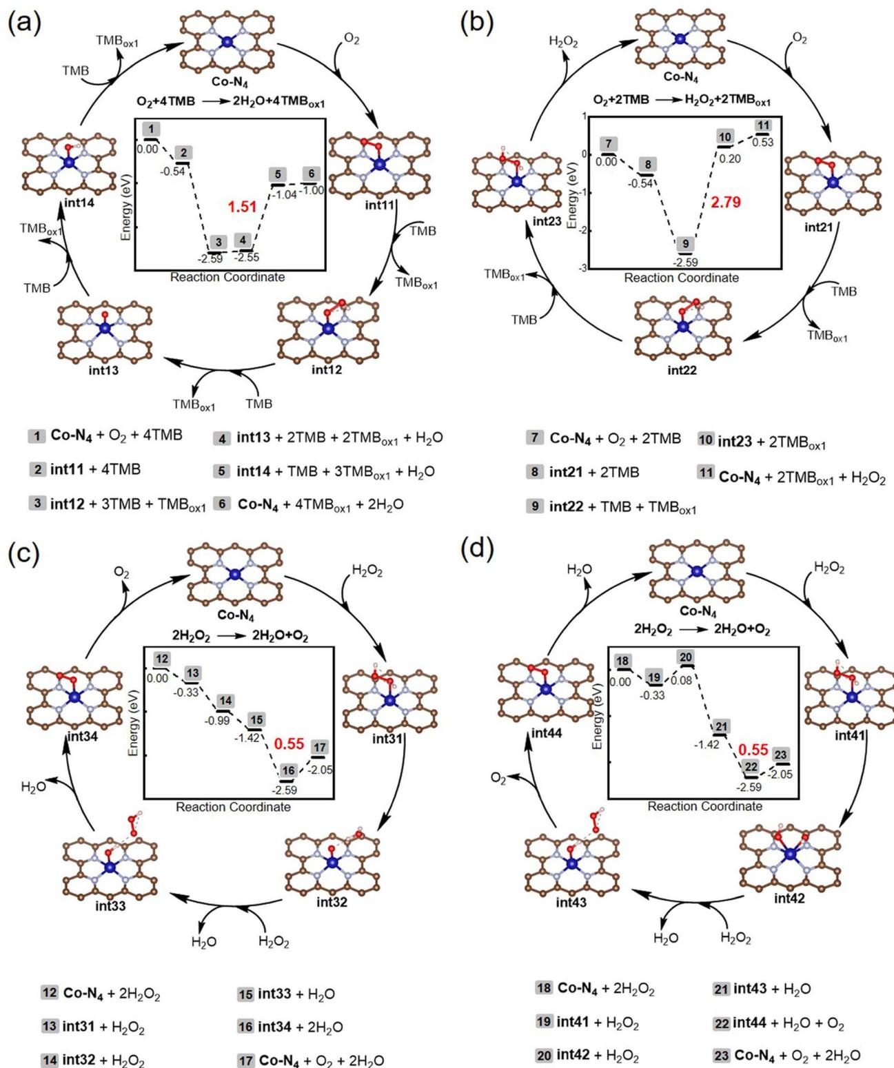
Fig. 3 Proposed mechanisms and calculated energy profiles for Co-N<sub>4</sub> centers. Four- (a) and two-electron (b) mechanisms for the oxidase-mimicking activities of Co-N-CNTs. Two possible catalytic mechanisms, corresponding to the heterolytic (c) and homolytic (d) cleavage of H<sub>2</sub>O<sub>2</sub>, for the catalase-mimicking activity of Co-N-CNTs. Chemical constituents of stationary points 1–23 are listed.
