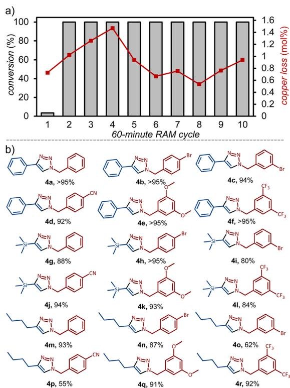
Fig. 2 (a) Conversion to **4a** compared to copper loss from the coil (in mol% with respect to **2a**) for 10 consecutive 60 minutes RAM cycles conducted using the same copper coil, based on quadruplicate measurements. (b) Substrate scope for herein developed RAM click-coupling reaction, with isolated yields indicated.
