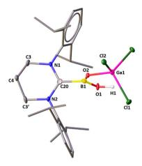
Fig. 3 The molecular structure of 3. Hydrogen atoms (except the hydrogens attached with oxygen atom) are omitted for clarity. Selected bond distances (Å), bond angles (deg), and torsion angle (deg): C20-N1 1.334(5), B1-C20 1.631(9), B1-O2 1.320(9), B1-O1 1.334(10), O1-H1 0.97(2), O2-Ga1 1.822(5), Ga1-Cl1 2.1803(14), Ga1-Cl2 2.159(2); N1-C20-N2 120.4(6), N1-C20-B1 119.7(3), O1-B1-O2 130.2(7), B1-O2-Ga1 131.1(5), Cl2-Ga1-Cl2 111.74(5).
