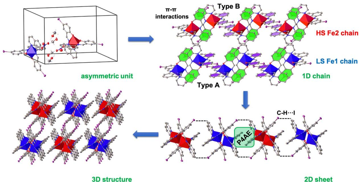
Fig. 3 Schematic illustration of the packing from the asymmetric unit to the final supramolecular 3D structure for **1** at 150 K (blue Fe1 centres, red Fe2 centres). This figure is intended as a guide to the discussion only.
