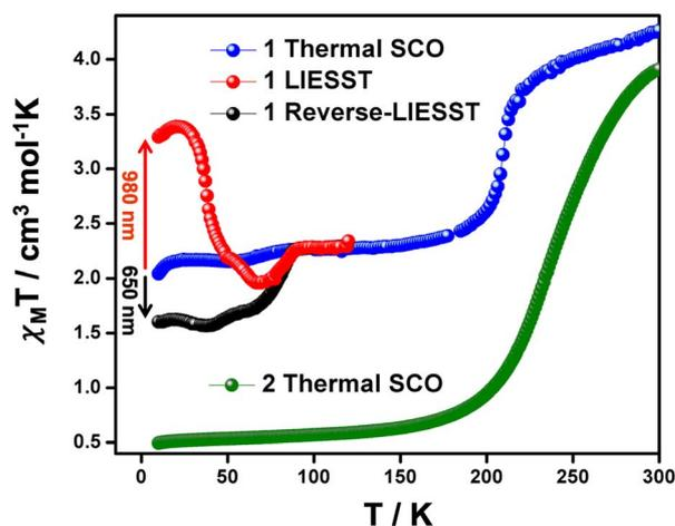
Fig. 5  $\chi_{\text{M}}T$  versus  $T$  plot (recorded at  $0.5 \text{ K min}^{-1}$ ) of 1 showing the thermal behaviour in the dark without any previous light irradiation (blue), after LIESST effect at 980 nm (red) and after reverse-LIESST effect at 650 nm (black) and thermal behaviour of 2 (green).
