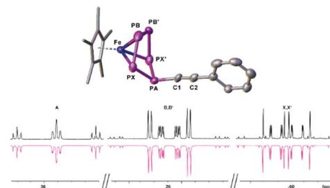
**Fig. 1** (Top) Solid-state molecular structure of **1c** with thermal ellipsoids at 50% probability level. Cations and hydrogen atoms are omitted for clarity, the  $\text{Cp}^*$  ligand is drawn in a wire frame model. (Bottom) Experimental (upwards) and simulated (downwards)  $^{31}\text{P}\{^1\text{H}\}$  NMR (161.98 MHz,  $\text{THF-d}_6$ ) spectrum of the anion of **1c**.
