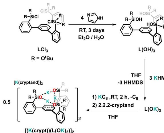
Scheme 1 Synthesis of the tripodal ligand **L(OH)<sub>3</sub>** and of the ligand radical salt  $[(\text{K}(\text{crypt}))(\text{L}(\text{OK})_3)]_2$ .
