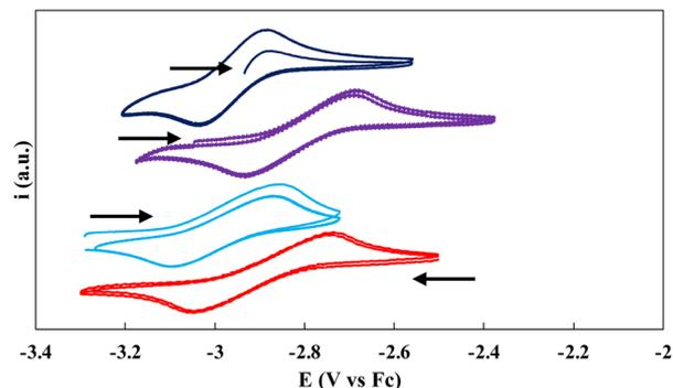
Fig. 4 Cyclic voltammograms of complexes **1** (red), **3** (blue), **5** (purple) and **5** + cryptand (dark-blue) in THF (0.1 M  $[\text{NBu}_4][\text{BPh}_4]$ ) at a 250  $\text{mV s}^{-1}$  scan rate versus  $\text{Fc}/\text{Fc}^+$  (arrows indicate the scan direction).
