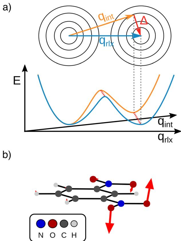
Fig. 7 (a) Schematic representation of the separable intrinsic ET coordinate (Marcus dimension,  $q_{int}$ , orange) and orthogonal structural relaxation ( $\Delta$ , red arrow) vs. the relaxed ET coordinate ( $q_{rlx}$ , blue) that may be obtained from a LICC approach. (b) Structural relaxation obtained by LICC between the second minimum at the Marcus dimension and fully optimized geometry.
