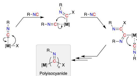
**Scheme 1** Generic mechanism for the polymerization of isocyanides. Note: an intermolecular process may also initiate the reaction, in which an external nucleophile attacks the carbon atom of a coordinated isonitrile ligand, generating the first propagating iminoacyl species.
