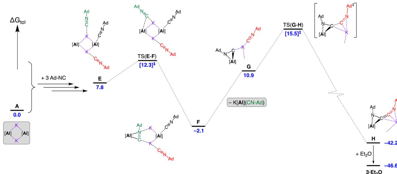
Fig. 10 Computed free energy profile (BP86-D3BJ(PCM =  $C_7H_8$ )/BS2//BP86/BS1 in  $\text{kcal mol}^{-1}$ ) for the dimerisation of Ad-NC at  $[K(Al(NON))]_2$  leading to formation of  $3 \cdot Et_2O$ . Note: charges and lone pairs on isocyanide groups omitted for clarity. See footnote ¶ and Fig. S28† for details of structures A–E.
