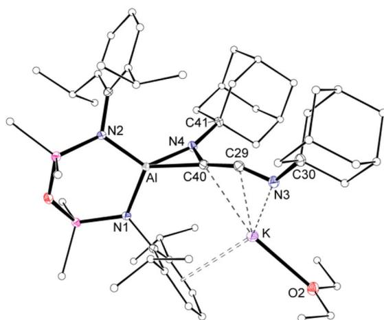
Fig. 5 Displacement ellipsoid plot (30%) of  $3 \cdot Et_2O$  (H-atoms omitted, peripheral carbon atoms represented as spheres). Selected bond lengths (Å) and angles (°) presented in Fig. 7.
