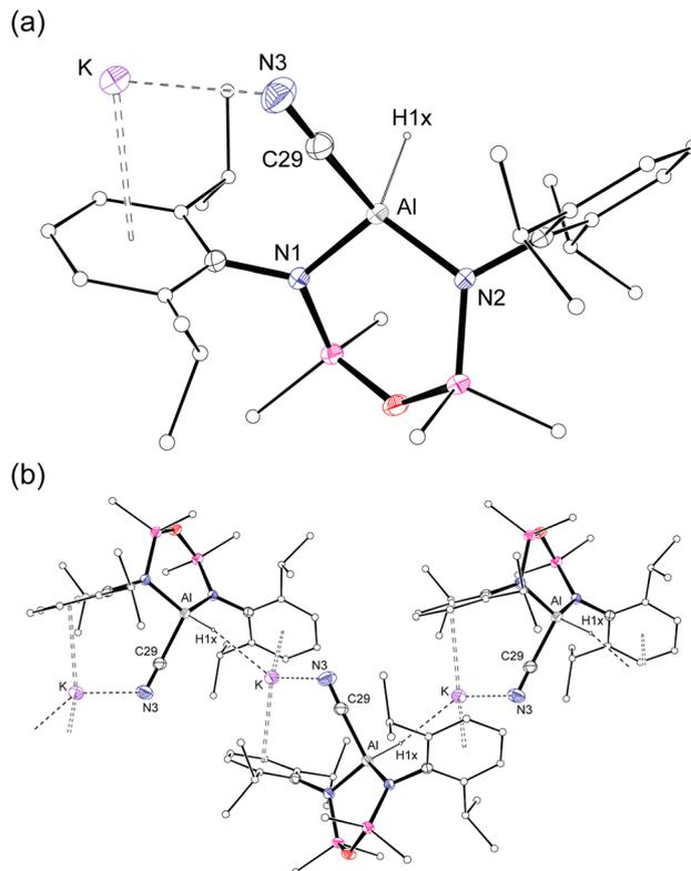
Fig. 2 (a) Displacement ellipsoid plot (30%) of the asymmetric unit of  $K[Al(NON)(H)(CN)]$  (**1a**). (b) Section of the 1-D chain formed by intermolecular  $K\cdots H$  and  $K\cdots N/C$  interactions.
