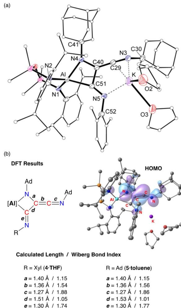
**Fig. 8** (a) Displacement ellipsoid plot (30%) of **4·THF** (H-atoms and disordered atoms omitted, peripheral carbon atoms represented as spheres). Selected bond lengths and angles presented in Table 1. (b) Summary of key bond parameters from DFT (BP86/BS2//BP86/BS1) and NBO analysis of **4·THF** and **5·toluene**, with a representation of the HOMO of **4·THF**.
