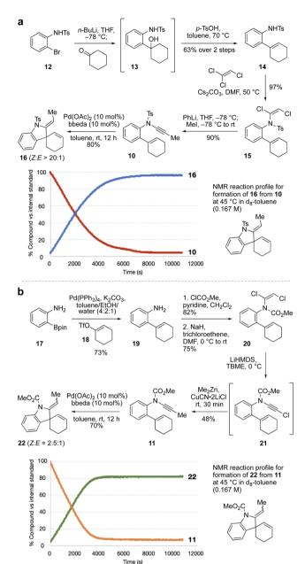
Scheme 2 Model spiro-ring synthesis (a), model fused-ring synthesis (b), and reaction kinetics.
