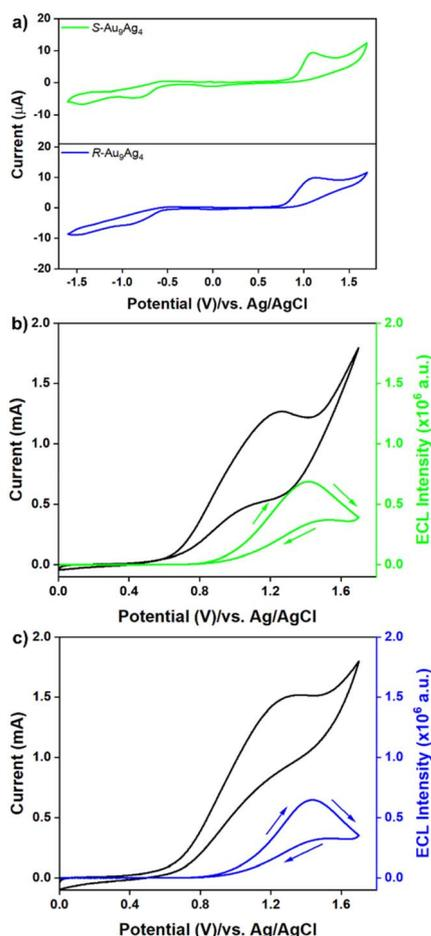
Fig. 3 (a) Voltammetric characterization of *R/S*-Au<sub>9</sub>Ag<sub>4</sub> in degassed DCM with 0.1 M tetrabutylammonium perchlorate (TBAP) as the supporting electrolyte. (b) and (c) CV (black curve) and corresponding ECL signal (blue/green curves) recorded in DCM containing 0.23 mM *R/S*-Au<sub>9</sub>Ag<sub>4</sub>, 700 mM TPrA, and 0.1 M TBAP. A platinum mesh electrode and Ag/AgCl wire were used as the working and reference electrodes, respectively. Scan rate = 0.1 V s<sup>-1</sup>.
