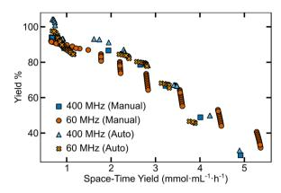
Fig. 3 Predicted Pareto fronts from low- and high-field NMR analysis outputs of manually and semi-automated processed data.
