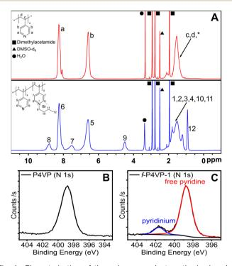
Fig. 4 Characterization of the polymer product synthesized under continuous flow. (A)  $^1$ H NMR spectra of P4VP (top, red) and f-P4VP-1 (bottom, blue) in DMSO-d<sub>6</sub>. (B). XPS N 1s spectrum of P4VP. (C). XPS N 1s spectrum of f-P4VP-1. Analysis reveals two distinct N species at 398.71 eV and 401.64 eV, corresponding to free pyridine and quaternized pyridinium on the polymer, respectively. Samples were isolated from solutions in DMAc prior to NMR and XPS analysis.
