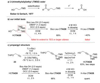
Scheme 12 Development of acid-resistant super silyl tags at the C-terminal (a) TMSE ester; (b) our initial tests of TAG8; (c) propargyl structure of TAG9.
