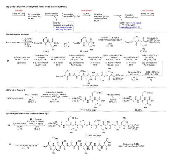
Scheme 11 Convergent synthesis of nelipepimut-S with Fmoc-chemistry (a) peptide elongation system; (b and c) preparation of two fragments; (d) convergent connection and removal of the tags.
