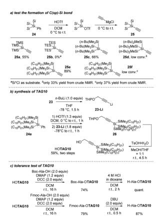
Scheme 13 Extension of the alkyl chains on the silicon atoms (a) test the formation of C–Si bond; (b) synthesis of TAG10; (c) tolerance test of TAG10.
