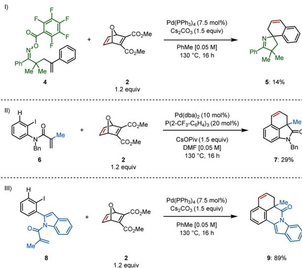
Scheme 4 Synthesis of analogous azacycles. (I) Spirocyclic pyrroline. (II) Dihydrobenzindolone. (III) Indolo[2,1-*a*]isoquinolinone. Reactions were performed on a 0.2 mmol scale; isolated yields are shown.
