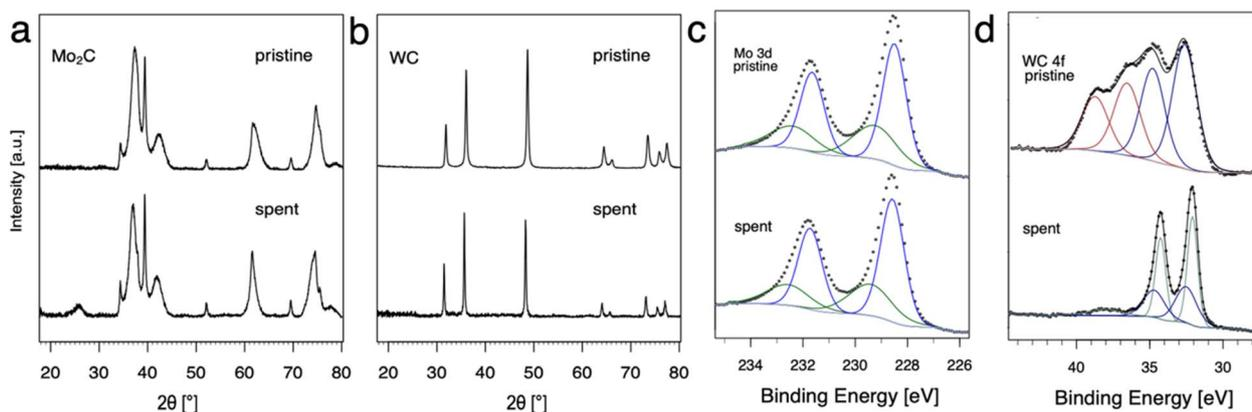
Fig. 2 Structural transformations for pristine and spent catalyst materials are shown. pXRD for (a)  $\text{Mo}_2\text{C}$ , (b) WC and XPS spectra of pristine and spent metal carbides: (c)  $\text{Mo } 3d$ , (d)  $\text{WC } 4f$ . The dots represent the recorded data and the solid lines show the results of a curve-fitting procedure.
