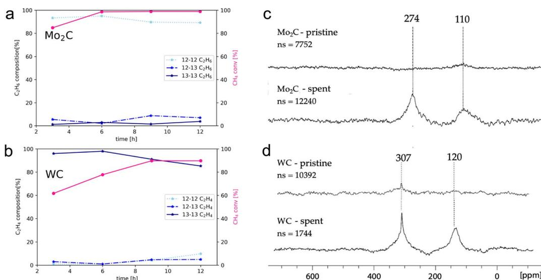
Fig. 3 Left: Product distribution for dilabelled, monolabelled and non-labelled  $\text{C}_2$  products in case of  $\text{Mo}_2\text{C}$  (a) and WC (b) as a function of contact time. Right:  $^{13}\text{C}$  MAS NMR characterization of pristine and spent (c)  $\text{Mo}_2\text{C}$  and (d) WC. The catalyst was contacted with 200 mbar  $^{13}\text{CH}_4$  (at r.t.) in batch for 24 h at 1100 °C (molar ratio 7.2 WC: 1  $^{13}\text{CH}_4$  and 6.9  $\text{Mo}_2\text{C}$ : 1  $^{13}\text{CH}_4$ ).
