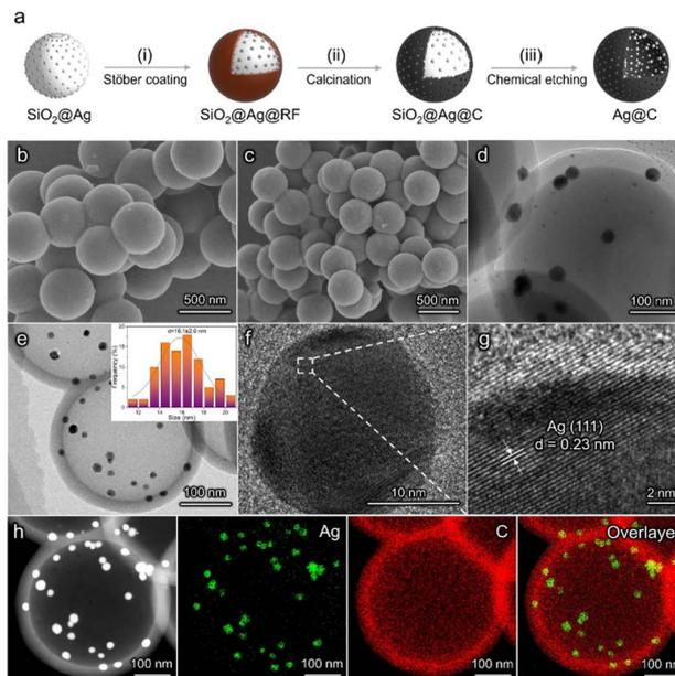
Fig. 1 Schematic illustration and morphological characterization. (a) Scheme of the synthesis process of the Ag@C catalyst. (b) SEM image of SiO<sub>2</sub>@Ag@RF. (c) SEM and (d) TEM images of SiO<sub>2</sub>@Ag@C. (e) TEM and (f and g) HRTEM images of Ag@C. The inset in (e) is the particle size distribution of Ag. (h) Energy-dispersive spectroscopy (EDS) elemental mapping images of Ag@C.
