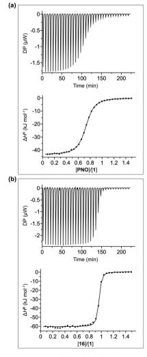
Fig. 4 ITC data for titration of (a) PNO (0.28 mM) into 1 (0.04 mM) and (b) 16 (0.28 mM) into 1 (0.04 mM) in water at 298 K. The raw data for each injection is shown (differential power, DP), along with the least-squares-fit of the enthalpy change per mole of guest ( $\Delta H^{\circ}$ ) to a 1:1 binding isotherm.
