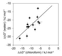
Fig. 9 The free energy contributions due to aromatic interactions in complex A ( $\Delta\Delta G^{\circ}$ ) measured using DMCs in water compared with the corresponding measurements in chloroform. The line of best fit is shown ( $R^2=0.49$ ).
