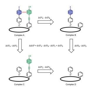
Fig. 2 Chemical double mutant cycle for evaluating the free energy contribution ( $\Delta\Delta G^{\circ}$ ) due to aromatic interactions with the blue ring of the guest to the overall stability of complex A. Only one of the four calix[4]pyrrole side-arms is shown for clarity, but the DMC measures the sum of interactions with four green aromatic rings on the host.
