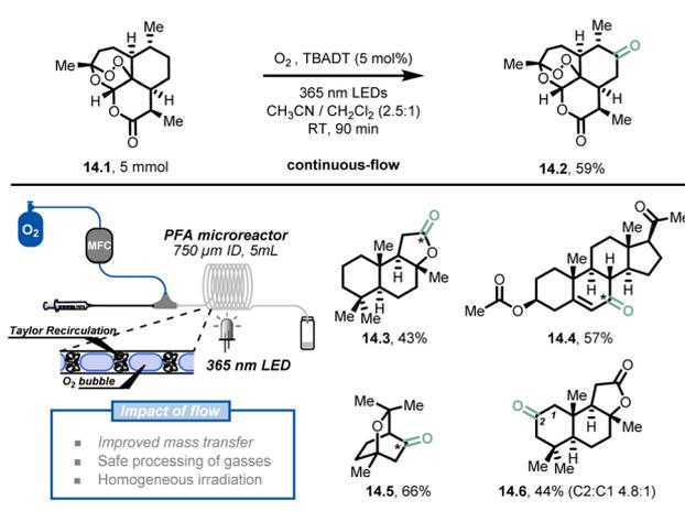
Fig. 14 Decatungstate-mediated C(sp<sup>3</sup>)-H oxidation with oxygen in continuous flow. TBADT: Tetra-*n*-butylammonium decatungstate. Reproduced from ref. 81 with the permission of Wiley-VCH, copyright 2018.
