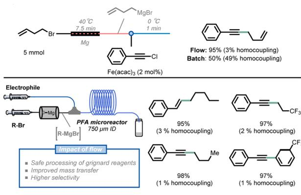
Fig. 5 Combining Grignard reagent synthesis with iron-catalyzed cross-coupling reaction in a telescoped flow process for C(sp)-C(sp<sup>3</sup>) bond formation.
