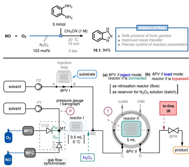
Fig. 15 Continuous-flow setup for the generation of N<sub>2</sub>O<sub>3</sub> and its subsequent use in synthetically-relevant contexts. CV: check valve; 6PV: six-position switch valve. MFC: Mass-Flow Controller. Reproduced from ref. 83 with the permission of Wiley-VCH, copyright 2022.
