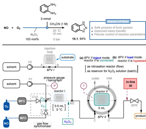
Fig. 15 Continuous-flow setup for the generation of N<sub>2</sub>O<sub>3</sub> and its subsequent use in synthetically-relevant contexts. CV: check valve; 6PV: six-position switch valve. MFC: Mass-Flow Controller. Reproduced from ref. 83 with the permission of Wiley-VCH, copyright 2022.
