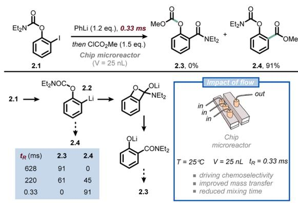
Fig. 2 Ultra-fast mixing provided by flow technology allows to outpace undesired anionic Fries rearrangement in the functionalization of iodophenyl carbamates at the *ortho* position.  $t_R$ : residence time.
